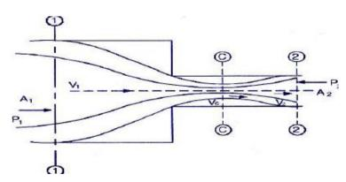
Using Bernoulli's equation, continuity and momentum equation at section 1-1 and 2-2, it can be proved that head loss due to sudden contraction is,
