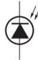
Fig. 1.18.1 Symbol of a photo diode
