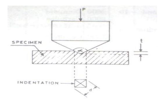
Fig.3.8.3(a) Square based pyramid indenter in Vicker's test
