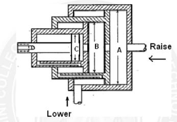
Since the diameter A of the ram is relatively large, this ram produces a large force for the beginning of the lift of the load. When ram A reaches the end of the stroke, ram B begins to move. Now ram B provides the required smaller force to continue raising the load. When ram B reaches the end of its stroke, then ram C moves outwards to complete the lifting operation. These three rams can be retracted by gravity acting on the load or by pressurized fluid acting on the lip of each ram.
