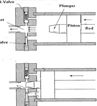
rate of deceleration is controlled. For starting the forward stroke of the piston, the fluid
