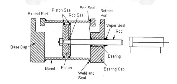
A rod wiper is provided at the end of the neck to prevent foreign particles and dust from entering into the cylinder along with the piston rod. When the fluid from the pump enters the cylinder through port 1, the piston moves forward and the fluid return to the reservoir from the cylinder through port 2. During the return stroke the fluid is allowed to enter the cylinder through port 2 and fluid from the other side of the piston goes back to the reservoir through port 1.
