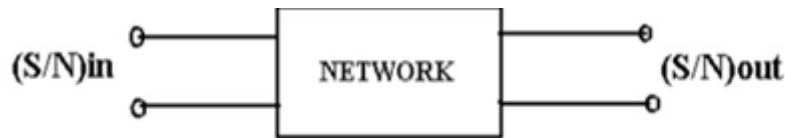
Figure 4.2.1 Block diagram for S/N Ratio
