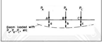
In most beam applications the strain energy, and hence the deflection, resulting from end loads and shear forces are taken to be negligible in comparison with the strain energy resulting from bending (torsion not normally being present),
