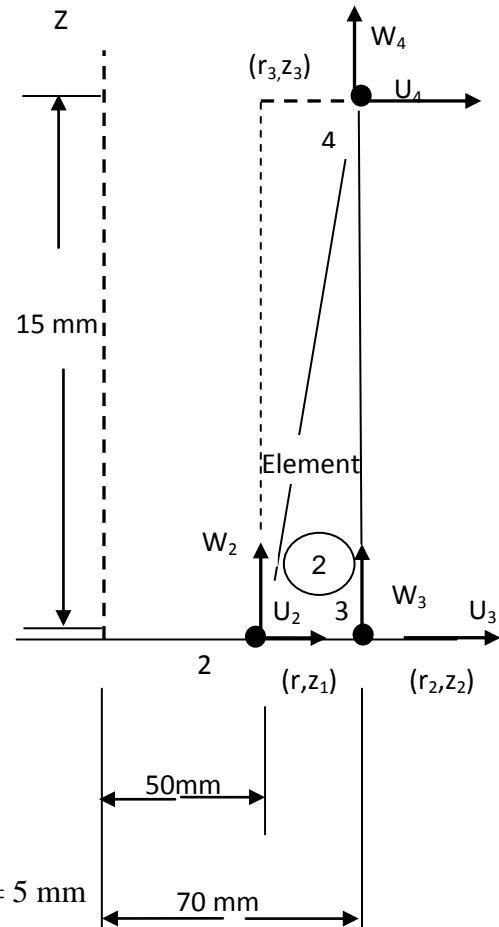
$$\text{Area of the triangle element} = \frac{1}{2} \times \text{Breadth} \times \text{Height}$$
