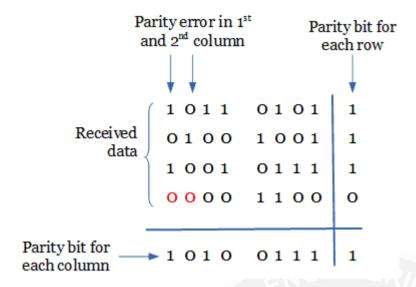
In the above figure, you can observe that there is no parity bit error for each row. But for the 1st and 2nd column the even parity is changed to odd parity, which is an error.
