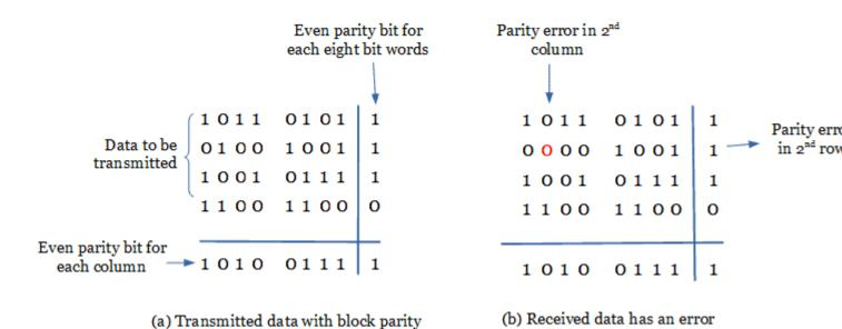
As shown above, even parity is given to each eight-bit word and for each column. In this case, the parity bit is called block parity. The block of data is transmitted from the
