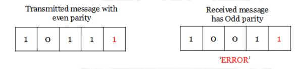
So, both even and odd parity codes are used only for the detection of error and not for the correction in the transmitted data. Even parity is commonly used and it has almost become a convention.
