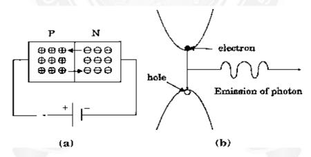
Fig:4.6.1 (a)semiconductor laser principle,(b)Emission of photon
