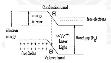
Fig 4.6.3. Energy band diagram
