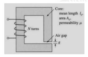
Assume that the core is of infinite permeability and neglect the effects of fringing fields at the air gap and leakage flux. (a) Calculate the reluctance of the core  $R_e$  and that of the gap  $R_g$ . For a current of i=1.5 A, calculate (b) the total flux  $\phi$ , (c) the flux linkages  $\lambda$  of the coil, and (d) the coil inductance L.
