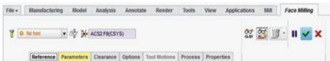
Fig. 3.25 Activated Face Milling dashboard in concise form
