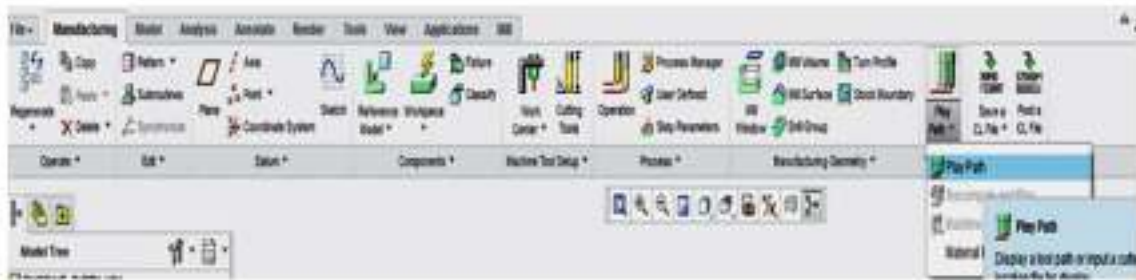
Fig. 3.29 Manufacturing ribbon toolbar with Play Path tab activated
