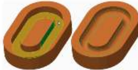
Figure 2 – Full Round Created by Selecting Three Surfaces
