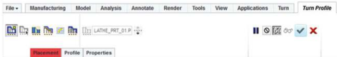
Fig. 10.17 Activated Turn Profile dashboard
