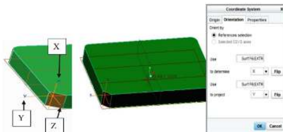
Fig. 2.56 Wrong orientation of X, Y and Z-axes of the Coordinate Systems
