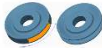
Figure 3 – Removing Material using a Revolve Feature
