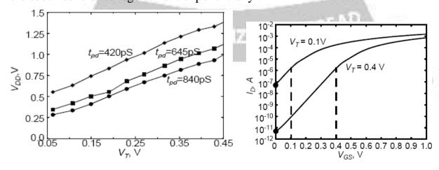
Figure: 2.5.3 Voltage Scaling (VDD/VT) on delay and leakage) (a) VDD/VT for fixed performance (b)
