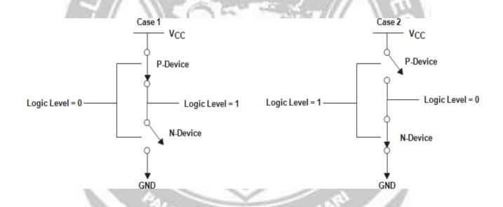
Figure 2.5.1: CMOS Inverter Mode for Static Power Consumption
