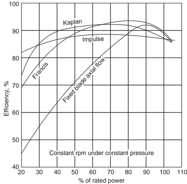
Figure 7.8.3 Load efficiency characteristics of hydraulic turbines
