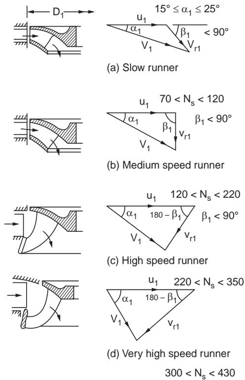
**Figure 7.7.3** Variation of runner shapes and inlet velocity triangles with specific speed
