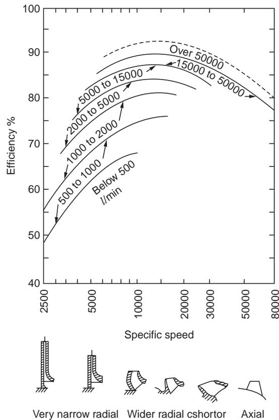
**Figure 7.3.2** Variation of efficiency and flow passage with specific speed.
