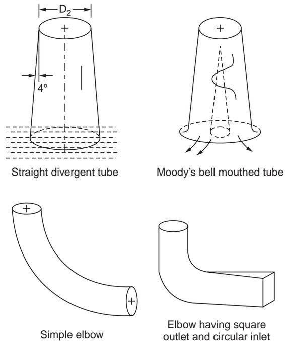
Figure 7.7.6 Various shapes of draft tubes
