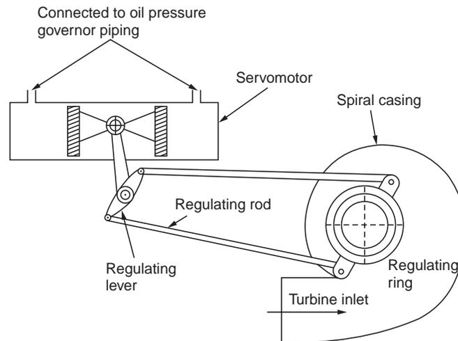
**Figure 7.9.2** Reaction turbine governor linkage
