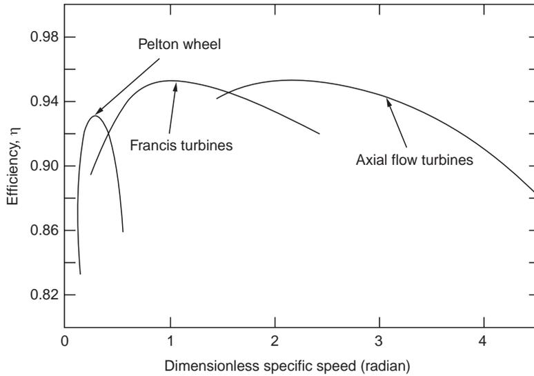
**Figure 7.3.1** Variation of efficiency with specific speed.
