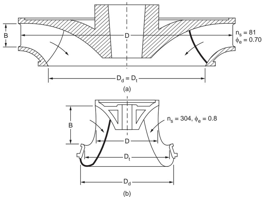
**Figure 7.7.4** Slow speed and highspeed runner shapes.
