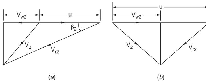
**Figure 7.6.6** Exit velocity diagrams for pelton turbine
