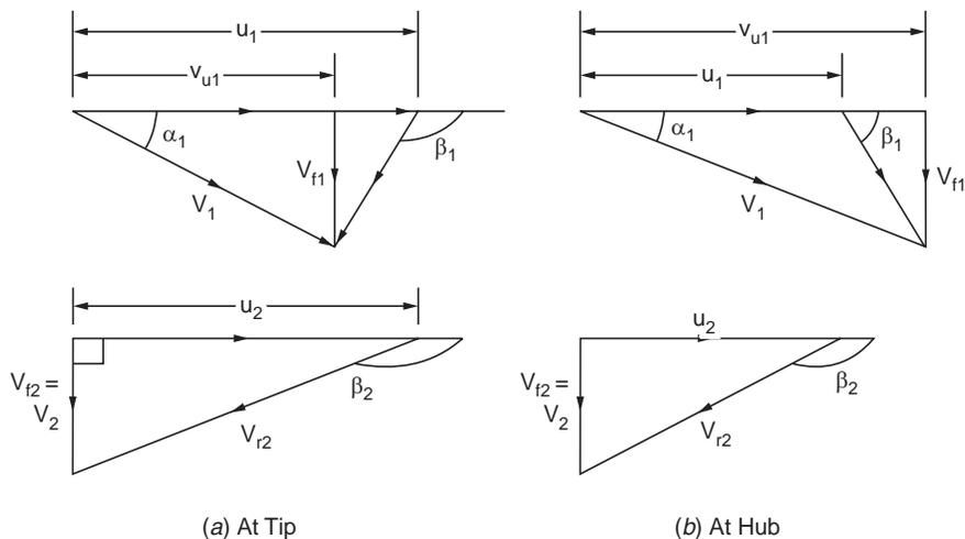
**Figure 7.8.2** Typical velocity diagrams for Kaplan turbine
