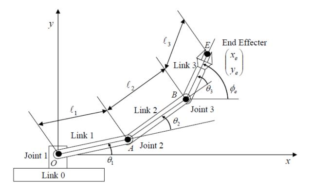
To describe this robot arm, a few geometric parameters are needed. First, the length of each link is defined to be the distance between adjacent joint axes. Let points O, A, and B be the locations of the three joint axes, respectively, and point E be a point fixed to the end-effecter.
