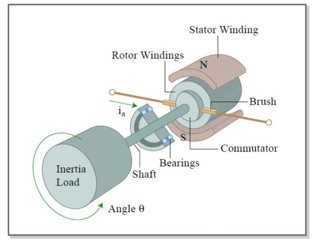
Figure 2.1.1 Construction of DC motor
