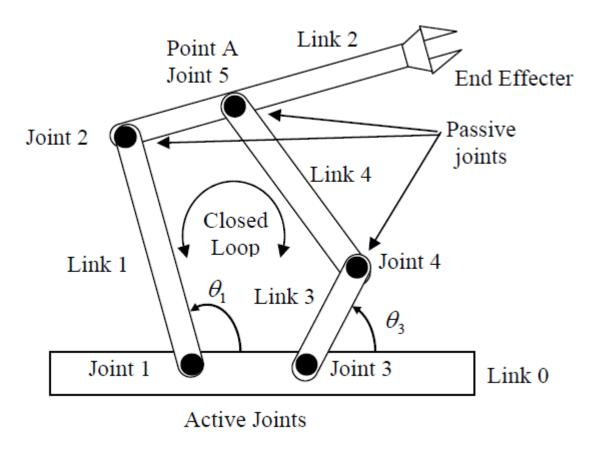
Figure 3.2.1 Five-bar-link parallel link robot
