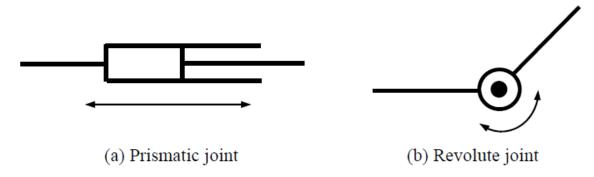
Combining these two types of primitive joints, we can create many useful mechanisms for robot manipulation and locomotion. These two types of primitive joints are simple to build and are well grounded in engineering design. Most of the robots that have been built are combinations of only these two types. Let us look at some examples.
