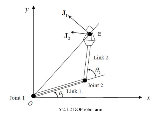
In general, each column vector of the Jacobian represents the end-effecter velocity and angular velocity generated by the individual joint velocity while all other joints are immobilized. Let be the end-effecter velocity and angular velocity, or the end-effecter velocity for short, and iJbe the i-th column of the Jacobian. The end-effecter velocity is given by a linear combination of the Jacobian column vectors weighted by the individual joint velocities.
