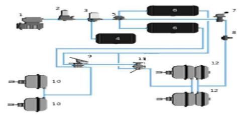
Highly simplified air brake diagram on a commercial road vehicle (does not show all air reservoirs and all applicable air valves). The air compressor is driven by the engine either by crankshaft pulley via a beltor directly from the engine timing gears. It is lubricated and cooled by the engine lubrication and cooling systems.
