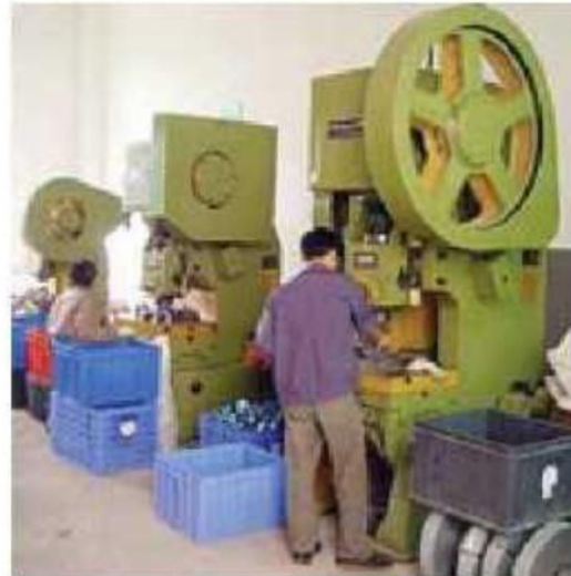
Punching press and flywheel.
