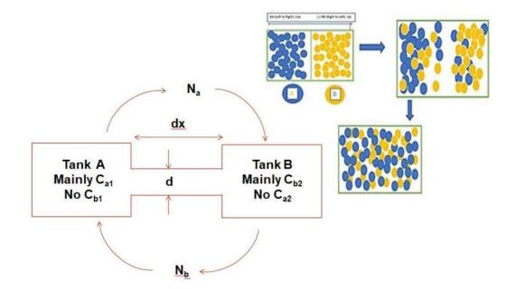
Type B: Steady State equimloar counter diffusion of a component "a" and "b"
