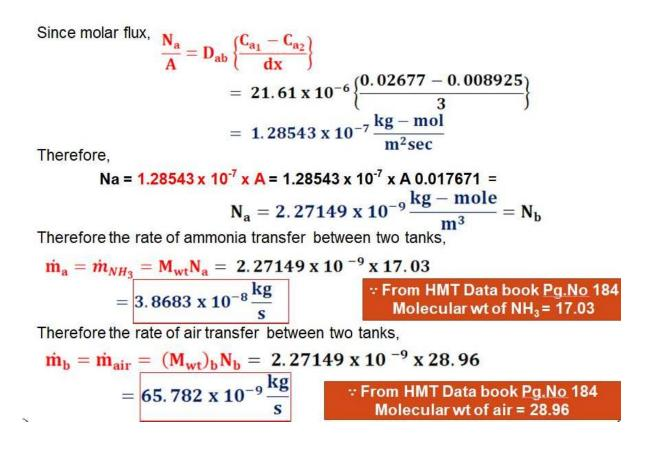
Type C: Steady State evaporation of a component "a" into a stagnant air
