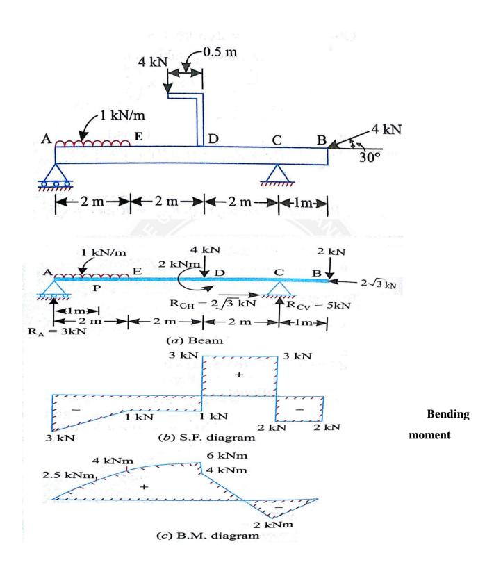
Calculation: [Sum of (Vertical force x Distance of load acting from required section)]
