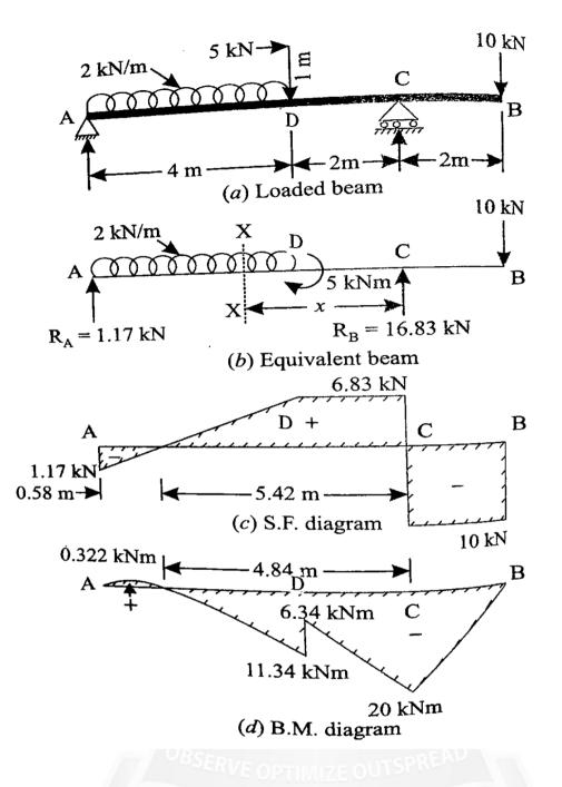
**Bending moment Calculation:** [Sum of (Vertical force x Distance of load acting from required section)]
