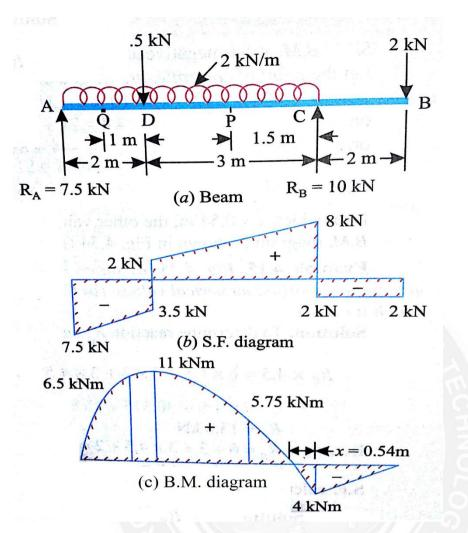
**Bending moment Calculation:** [Sum of (Vertical force x Distance of load acting from required section)]
