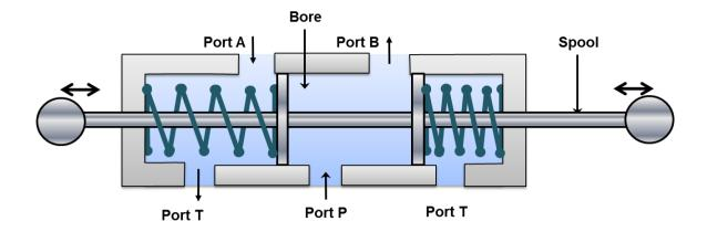
When left end (port B) is actuated, the port P is connected with ports B and T is connected with port A as shown in Figure 5.5.1. Similarly, when the right end is actuated the port P is connected to A and working port B is connected to port T as shown in FigureThe three position valves are used when the actuator is needed to stop or hold at some intermediate position. It can also be used when the multiple circuits or functions are accomplished from one hydraulic power source.
