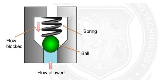
required. These valves can wear out or can generate the cracks after prolonged usage and therefore they are mostly made of plastics for easy repair and replacements.
