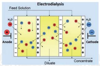
Water is handed between a negative electrode and a high-quality electrode. Ion exchange membranes permit solely high-quality ions to transfer toward the negative electrode from the feed water and negative ions to the positive electrode.
