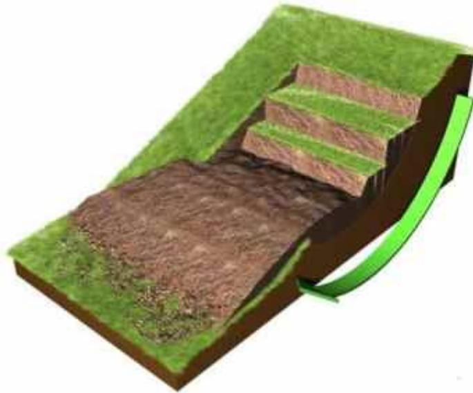
Fig 5.3: Rotational Failure
