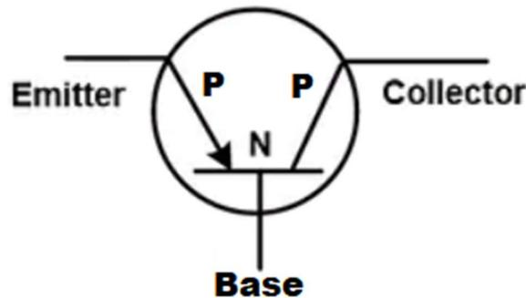
**Fig:2.2.1 Symbol of PNP Transistor**
