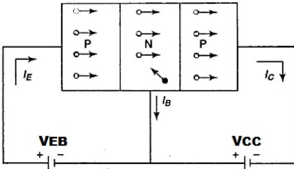
**Fig:2.2.3 Working Principle of PNP Transistor**
