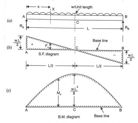
First to find the reaction force at A and B as  $R_A$  and  $R_B$  by the two steps are followed. Step1: Take moment about A = 0  $\gg$   $R_B \ge L - w.L \ge \frac{L}{2} = 0 \gg R_B = \frac{WL}{2}$ Step2: Sum of upward force = Sum of downward force  $\gg R_A + R_B = W.L$
