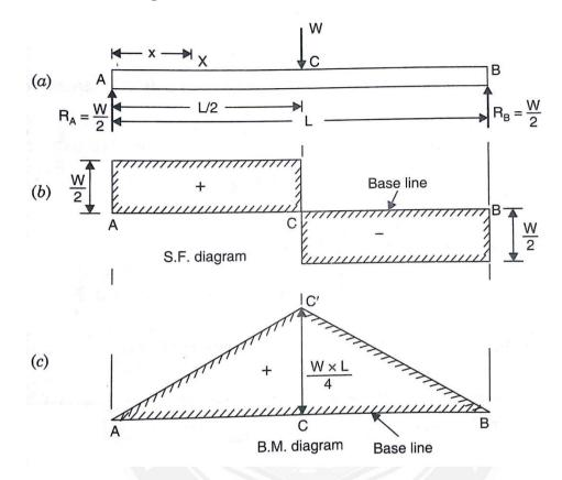
First to find the reaction force at A and B as  $R_A$  and  $R_B$  by the two steps are followed. Step1: Take moment about  $A = 0 \gg R_B \ge L - W \ge \frac{L}{2} = 0 \gg R_B = \frac{W}{2}$ Step2: Sum of upward force = Sum of downward force  $\gg R_A + R_B = W$
