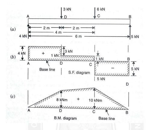
**Bending moment Calculation:** [Sum of (Vertical force x Distance of load acting from required section)]
