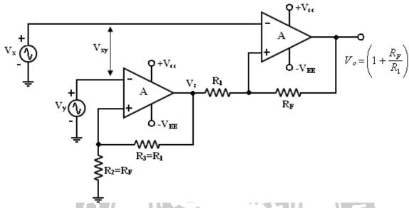
By finding the gain of these 2 stages, we can obtain the overall gain of the circuit, The o/p
