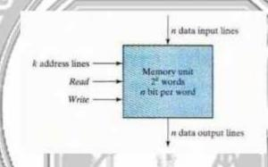
The memory unit is specified by the number of words it contains and the number of bits in each word. The address lines select one particular word. Each word in memory is assigned an identification number, called an address, starting fro 0 to  $2^k - 1$ , where k is the number of address lines. The selection of a specific word inside memory is done by applying the k- bit address to the address lines.
