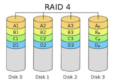
Each entire block is written onto a data disk. Parity for same rank blocks is generated on Writes, recorded on the parity disk and checked on Reads. RAID Level 4 requires a minimum of 3 drives to implement.
