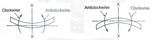
Similarly the bending moment at a section is considered negative if the bending moment at that section is such that it tends to bend the beam to a curvature haling convexity at the top. The negative B.M. as hogging Moment.
