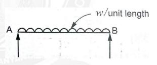
For numerical problem solving, the total UDL is converted into a point load acting at the centre of load.
