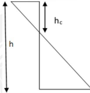
In clay under undrained condition at climatic temperature variation and due to water drain in season's soil volume shrinkage, cause compression due to soil self weight, surcharge and live load, cause tensile stress and spilt or fracture in the clay mass especially.
