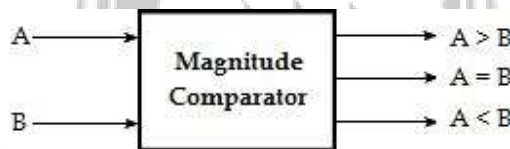
Fig : 2.21 - Block diagram of magnitude comparator
