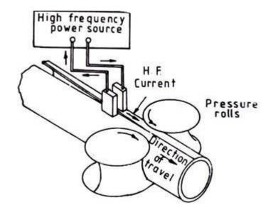
Figure shows a high frequency resistance welding setup for tube production. As shown, the two contact blocks are placed on opposite sides of the V- shaped gap and the current flows through the shortest path between the contacts and concentrates entirely at the edges of the metal. As the process employs a high voltage of about 100 volts, no difficulty is encountered in achieving good electrical contact between the contact blocks and the metal even when the material has oxide scale on it.
