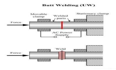
It is a resistance welding process that produces coalescence over the entire area of faying surfaces or progressively along a butt joint by the heat obtained from the resistance to the flow of welding current through the area where those surfaces are in contact. It can be used only if the parts to be welded are equal in cross-sectional area.
