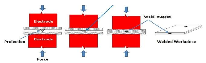
You can see in the above image that the projection means the embossed joints are formed on one of the base metals and then, these base metals are kept in between the two electrodes and force is applied perpendicular to the electrodes.
