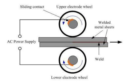
In seam welding a rather complex control system is required. This involves the travel speed as well as the sequence of current flow to provide for overlapping welds. The welding speed, the spots per inch, and the timing schedule are dependent on each other. Welding schedules provide the pressure, the current, the speed, and the size of the electrode wheels.
