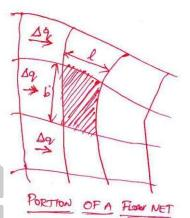
$\Delta q =$  discharge passing through the flow channel
