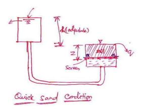
When the soil particles are in the state of critical equilibrium,
