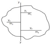
$$I = m_1 r_1^2 + m_2 r_2^2 + m_3 r_3^2 + \dots$$
