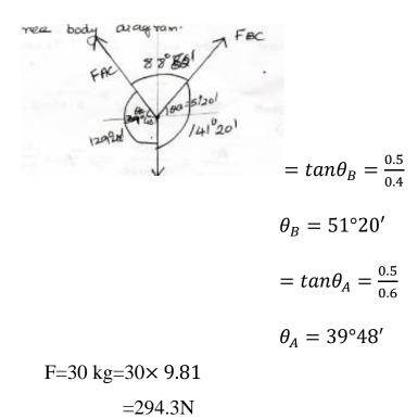
$$\frac{F_{AC}}{\sin 141^{\circ}20'} = \frac{F_{BC}}{\sin 129^{\circ}48'} = \frac{294.3}{\sin 88^{\circ}52'}$$
