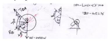
No of force is 3, so by using Lami's theorem
