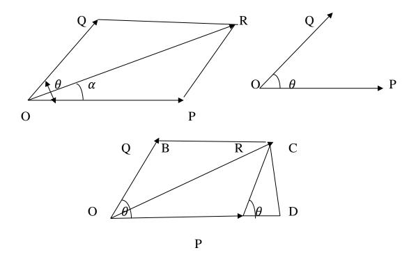
Let pand Q are two concurrent force acting on a point O at an angle of  $\theta$ .
