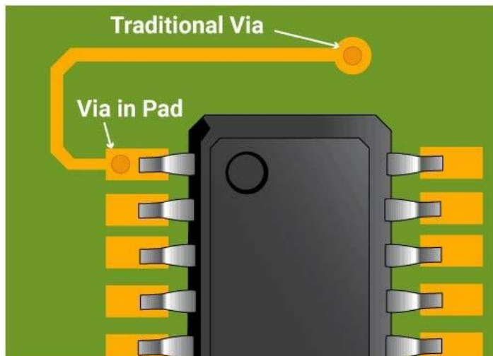
Via-In-Pad Vs. Traditional Via
