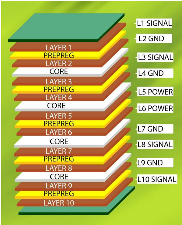
10-layer stackup with signal layers
